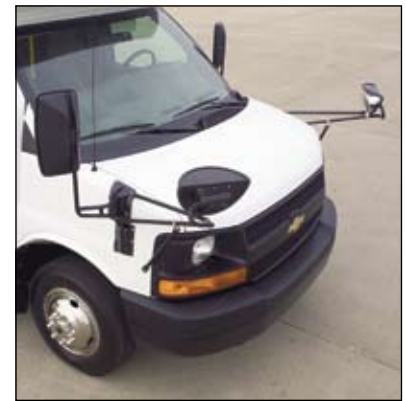
Front 7" x 14" flat & 6" x 3.5" convex mirrors with left and right cross-view mirrors
